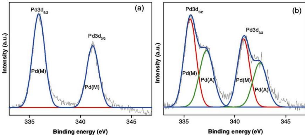
**Figure 4.** Core level spectra of Pd ( $3d_{5/2}$  and  $3d_{3/2}$ ) at temperatures of (a) 25°C, (b) 400°C, respectively. Peaks Pd (M) and Pd (A) corresponds to Pd metal and Pd alloy.
