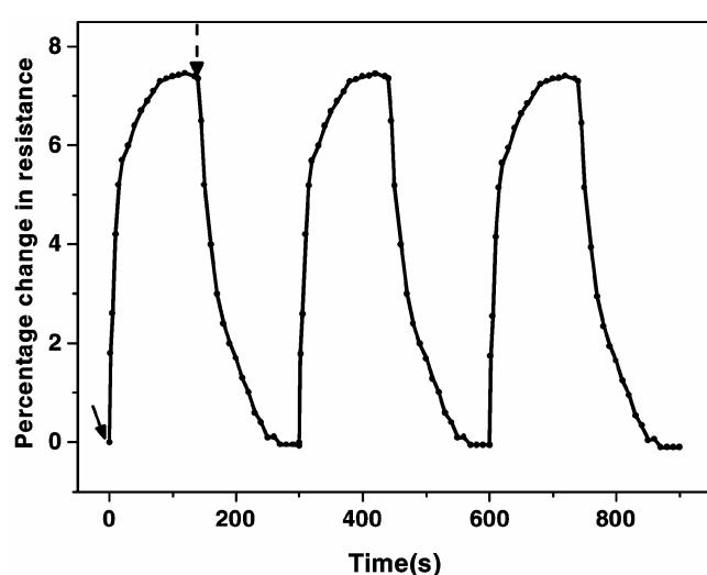
**Figure 1.** Stable and reversible hydrogen sensing response of Cu/Pd bimetal layers. Solid and dotted arrows show loading and deloading points.
