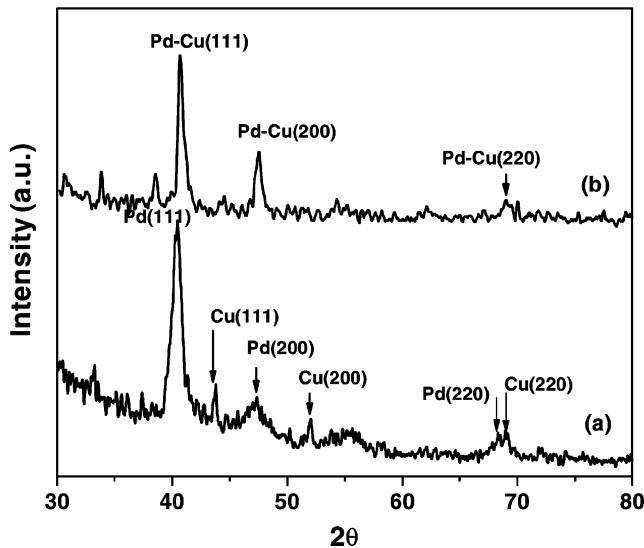
**Figure 5.** X-ray diffractograms of (a) as-deposited and (b) 400°C annealed Cu/Pd bimetal layers.
