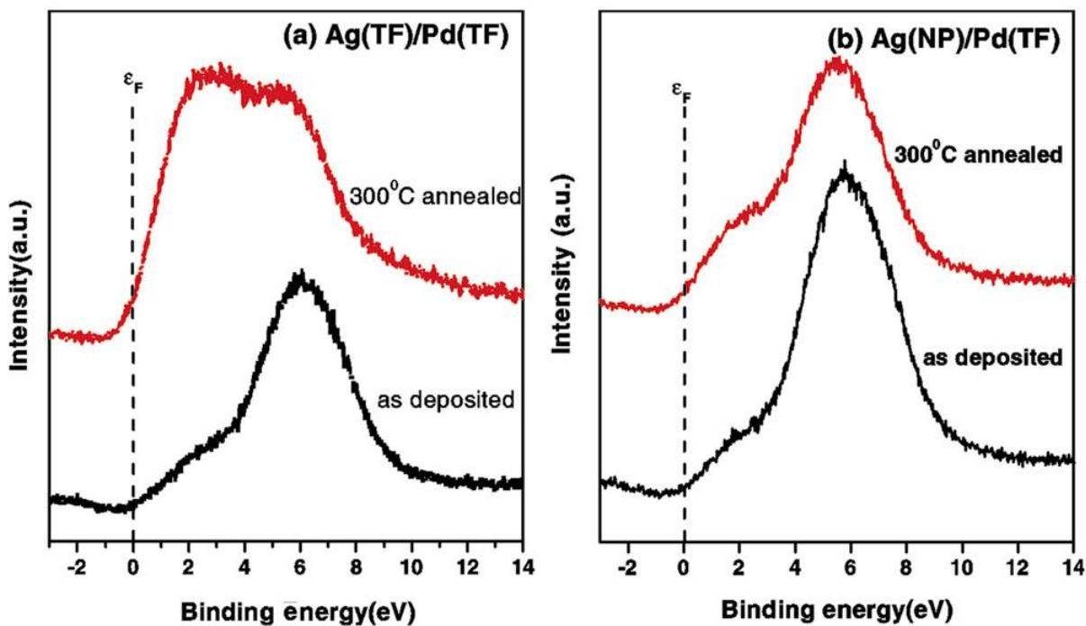
**Figure 7.** Valence band spectra of as-deposited and 300°C annealed (a) Ag(TF)/Pd and (b) Ag(NP)/Pd(TF) samples.
