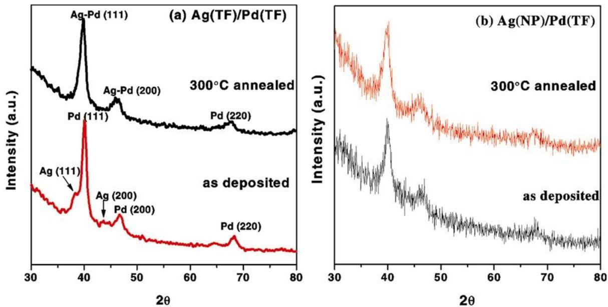
**Figure 6.** X-ray diffractograms of as-deposited and 300°C annealed (a) Ag(TF)/Pd(TF) and (b) Ag(NP)/Pd(TF) samples.
