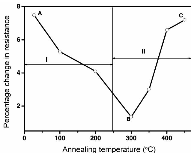
**Figure 2.** Hydrogen sensing response of Cu/Pd bimetal layer at 100% H<sub>2</sub> concentration and at different annealing temperatures.
