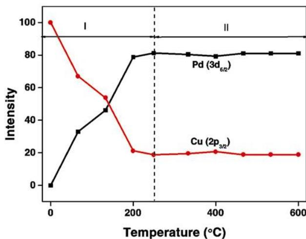
Figure 3. Area of Pd ( $3d_{5/2}$ ) and Cu ( $2p_{3/2}$ ) core level peaks as a function of annealing temperature. Regions I and II corresponding to figure 2 are also shown.
