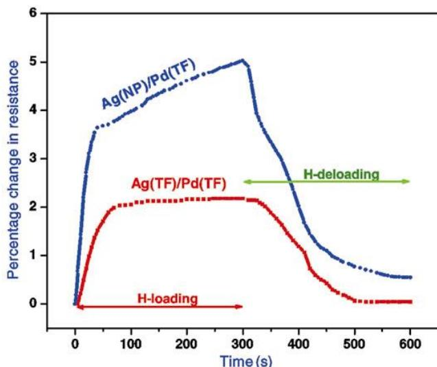
**Figure 8.** Hydrogen sensing response of 300°C annealed Ag(TF)/Pd(TF) and Ag(NP)/Pd(TF) samples.
